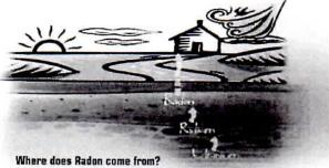
Radon comes from the soil. It is produced by the natural decay of uranium and radium commonly found in nearly all soils in Minnesota. As a gas, radon moves freely through the soil and eventually into the air you breathe. Our homes tend to draw soil gases, including
